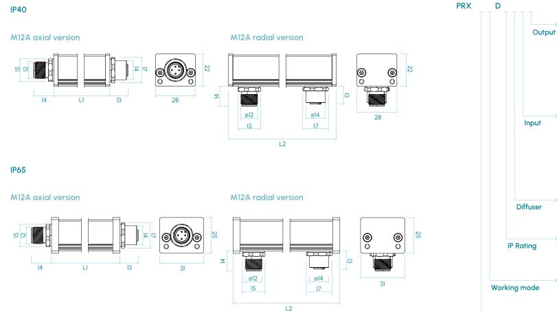
YL - M12A radial female connector Output PY - 10 cm axial cable with M12A female connector **RY** - 10 cm radial cable with M12A female connector Κ - Axial Cable, 2 m KL - Radial Cable, 2 m - M12A axial male connector YL - M12A radial male connector PY - 10 cm axial cable with M12A male connector RY - 10 cm radial cable with M12A male connector - Semidiffuse С U - Ultradiffuse - IP40 3 - IP65 5 P - Power Е - Eco D - Dual: Power/Eco 1 - 18 - 75 mm steps Length
